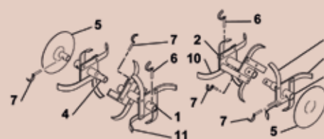
3 - Standard tool 135: 06726-732-003HE Hexagonal shaft 23 mm
